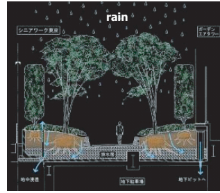
Rainwater infiltrates the underground and use for evaporation cooling
