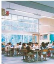
Ordinary Classrooms have Large Windows. Light Shelf guides light to the Interior.
